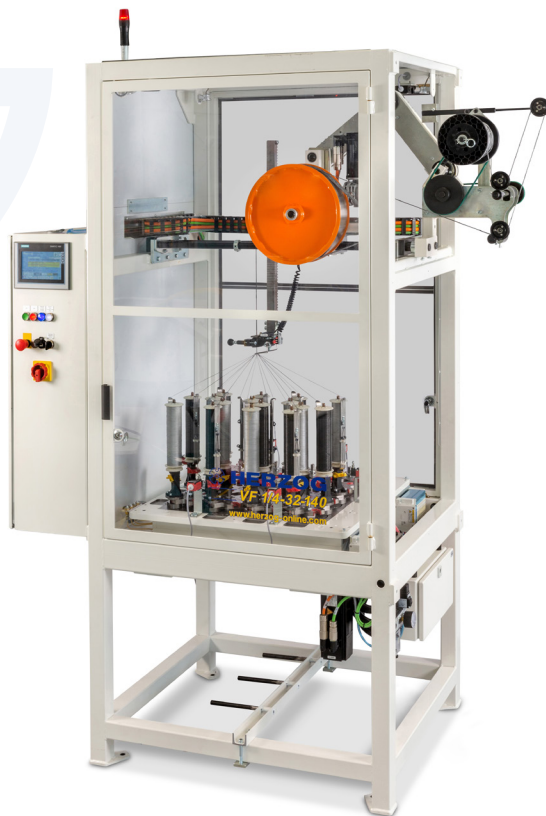
Variation braider VF 1/4-32-140 to produce braids with carrier numbers between 4 and 32
