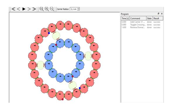
CAB Soft helps to create and simulate step sequences for all advanced Herzog braiding machines
